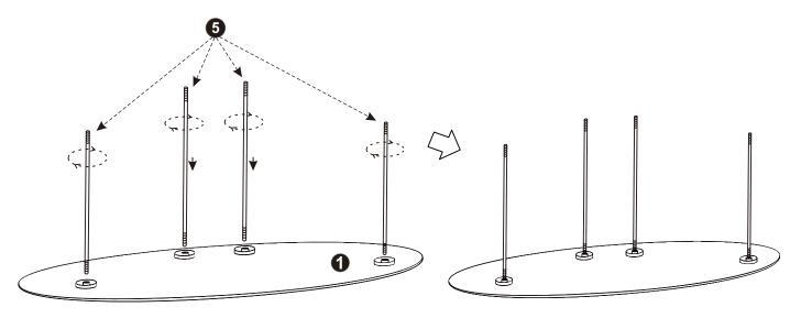
**Step 2**•Insert 4X table stand tube(3) and 4X plastic washer(6) through screw rod (5).
